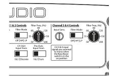
1) "Filter Mode" Control: The A4300 employs a 12dB per octave filter for each pair of channels (one filter for channels 1&2 and another filter for channels 3&4). Each of these filters can be configured independently into one of two filter types or defeated completely by way of the three-position "Filter Mode" switches:
